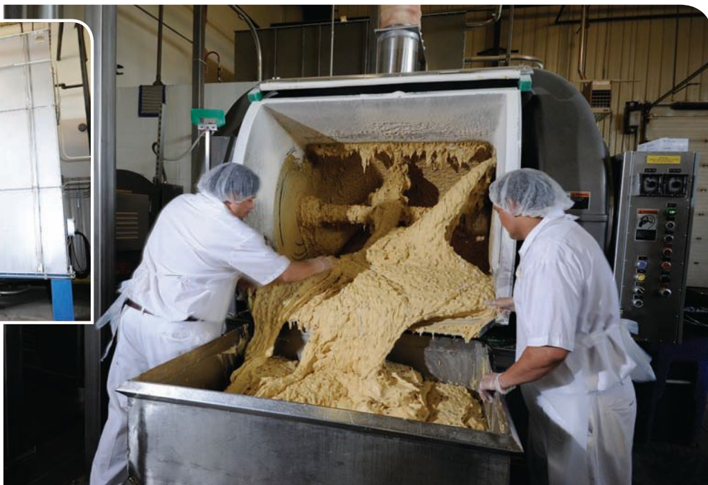
Above, an indoor flour silo with a maximum capacity of 100,000 lb. was recently added to the plant. Right, line operators empty the biscotti dough from a spiral mixer to a trough.
