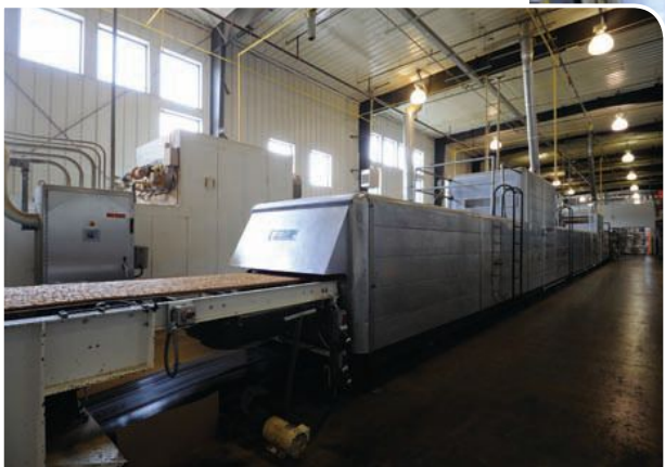
Below left: The massive, 110-ft.-long, first-bake tunnel oven really 'cooks' during the company's super-busy fall season, when the plant runs 24 hours a day and sometimes six days a week. Right, almond biscotti dough is topped with ground almonds and sprayed with an egg wash before it's baked the first time. The dough bakes twice, hence the 'biscotti' name.
