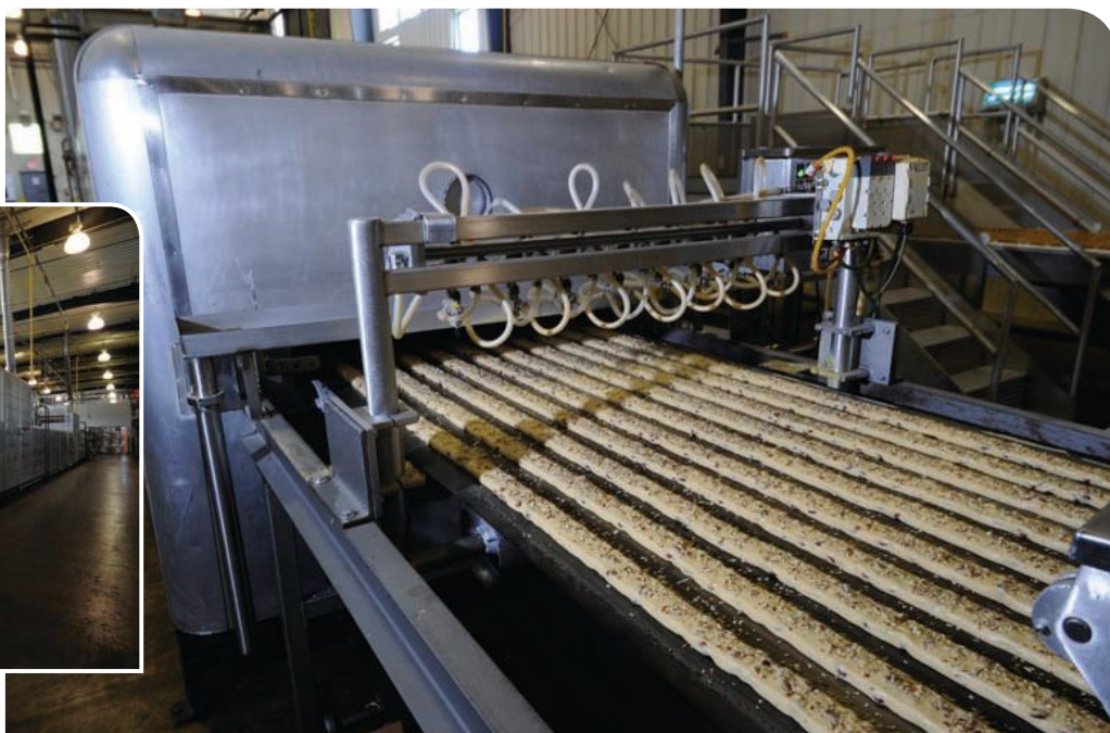
Below left: The massive, 110-ft.-long, first-bake tunnel oven really 'cooks' during the company's super-busy fall season, when the plant runs 24 hours a day and sometimes six days a week. Right, almond biscotti dough is topped with ground almonds and sprayed with an egg wash before it's baked the first time. The dough bakes twice, hence the 'biscotti' name.
